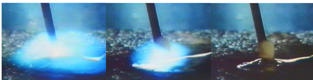
Fig. 19: Mod de transfer prin arc scurt
