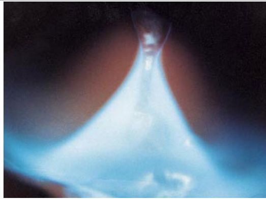
Fig.21: spray arc transfer mode
