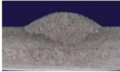
Fig. 16: welding with He
