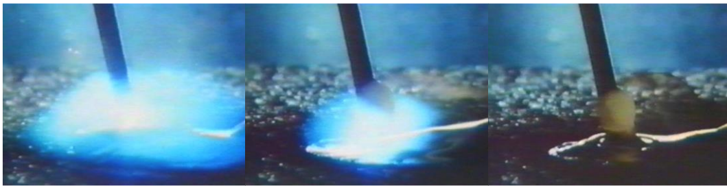
Fig.19: short arc transfer mode
