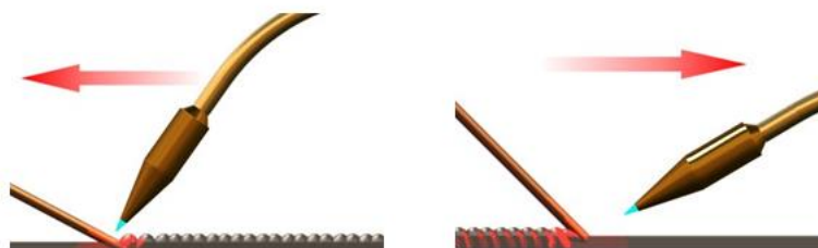
Fig. 4.1: welding techniques (leftward, on the left and rightward, on the right)
