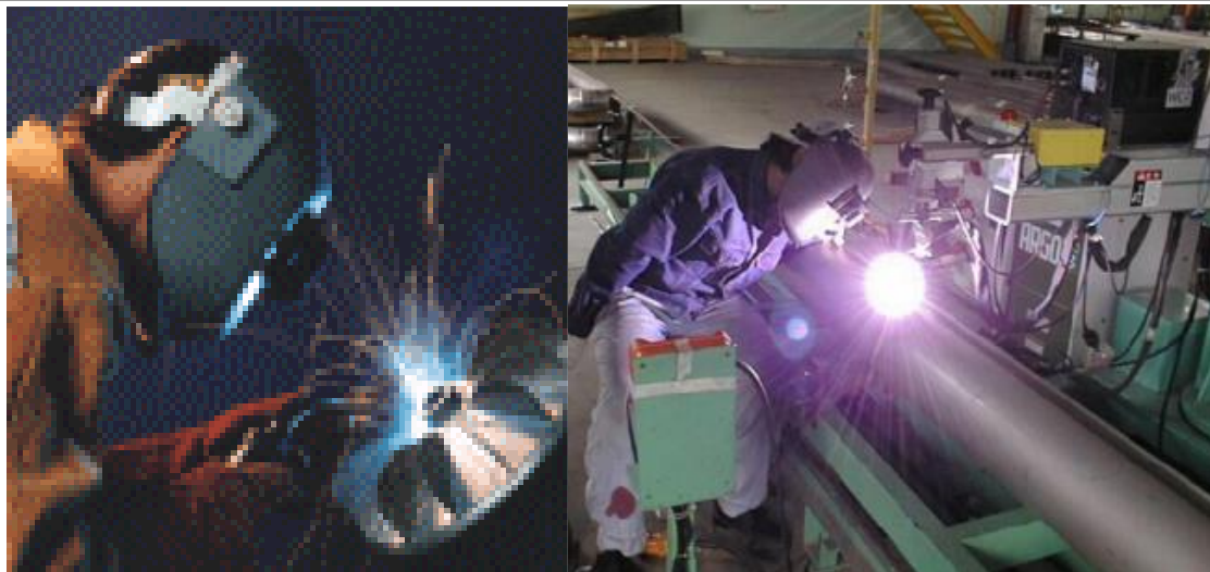
Fig.3: partly mechanized and fully mechanized welding
